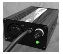
When the yellow LED on the motorcycle and the green LED light up on the charger means that that the Battery too warm or too cold for loading is.
