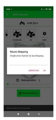
Adjust the values accordingly and press SEND to send the set parameters to the motorcycle. The display starts to flash and the motorcycle switches off after the data has been successfully transmitted. The new parameters are activated from the next start.
