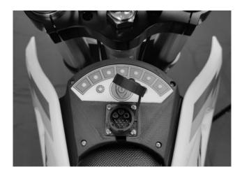
▷ Connect the charging plug of the charger to the charging connection of the motorcycle (bayonet lock), charging now begins automatically and the LED on the HVR charger lights up red.
